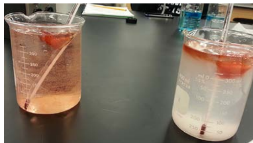
Figure 1: Left: Red ice-cube melting in DI water. Right: Red ice cube melting slower in salt water.
