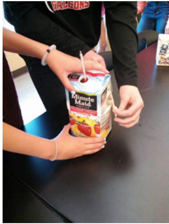
Figure 3. Assembling the milk carton house around the bottle of hot water. Note the thermometer sticking out of the "chimney."
